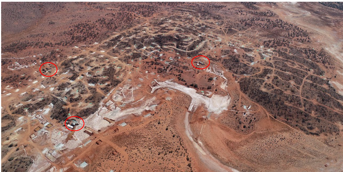
Plate 1 – Apollo Hill resource area, three RC drill rigs and expanding drill pattern – Photo taken 11 September 2020
