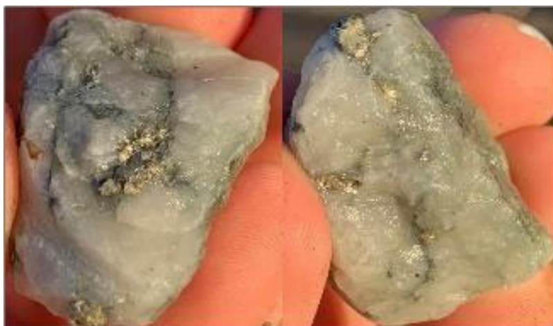
Plate 3 – Cave in material from historical 1.4m drive intercepted in WWDD0002 - Mineralised quartz veins at 334.9m – Graded at 1.22g/t Au
