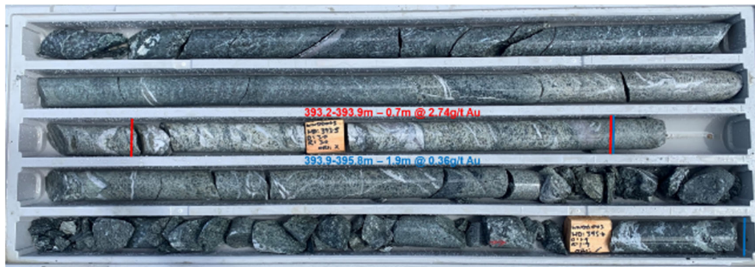
Plate 1 – Hole WWDD0003 Silica – Sericite - Pyrite Alteration, Quartz Veining and Ductile Shearing/Strain within Diamond Drill Core
