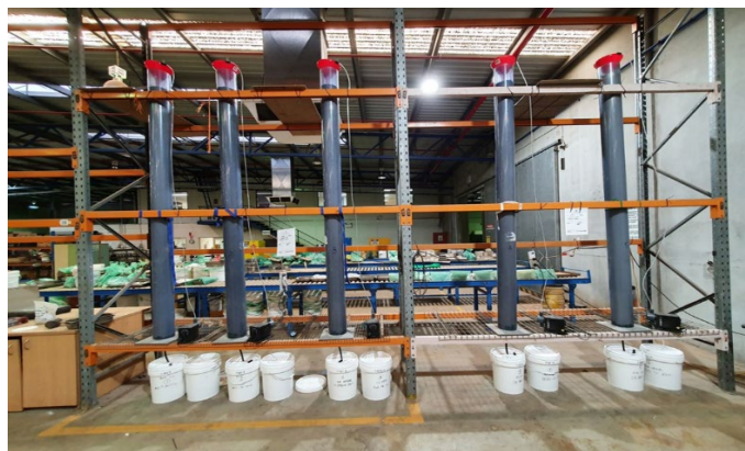
Plate 1 – Apollo Hill Heap Leach column tests underway at Bureau Veritas in Canning Vale (March-April 2022). The tests are being performed across a range of rock types and gold grades and crushing techniques to assess leaching kinetics (speed and efficiency) and scalability.
