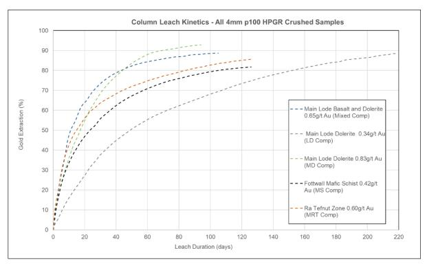
Figure 4: Column Leach Recovery Test Curves 4 mm P100 HPGR – strong leach kinetics – a predictable narrow band of recovery results.
