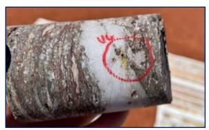
Plate 2: AHDD0018 (0.6 m @ 333 g/t Au from 20.2 m) - visible gold in quartz veins - HQ3 core
