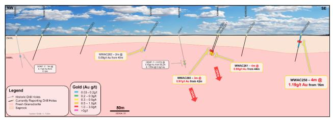
Figure 6: Long Cross Section of Saturn Metals 'Pioneer' Prospect. Historical hole traces seen in grey and recently reported intercepts in white.
