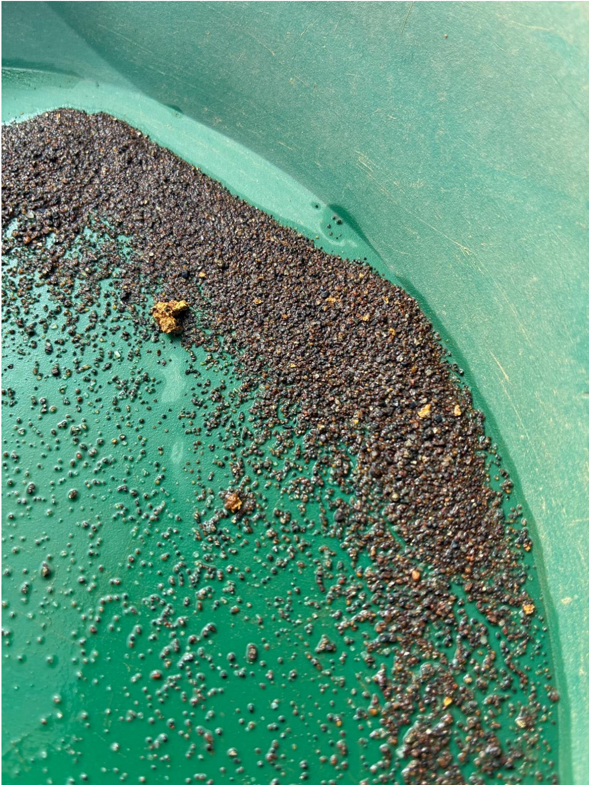
Plate 1 — AHRC1581 Drill Spoil Gold Pan — 1m @ 277g/t Au — 55-56m — Coarse visible gold present throughout the pan.
