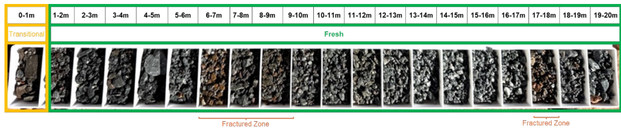
Plate 2 – Typical Weathering Profile – Apollo Hill - Main Lode – AHRC1148 RC Chips (Fresh basalt rock from 1m)
